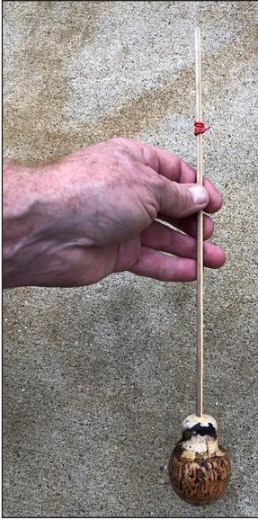
Figure 7. Homemade water level gauge.
