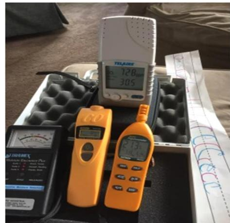
*We use a variety of meters to gauge moisture and ventilation during IAQ checks.*
