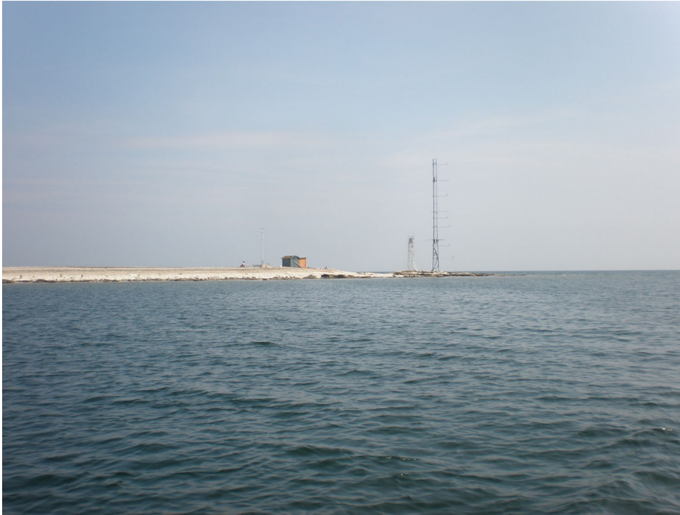
Fig. 2. The two towers at the Östergarnsholm station (facing east). The 30 m high tower is for flux and meteorological measurements, and the 10 m high tower for aerosol measurements.
