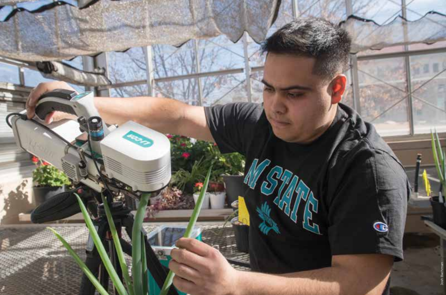
Gomez uses an Li-6800 photosynthesis gas exchange instrument to take photosynthetic measurements of an onion's leaves as part of a project examining photosynthetic rates of onions grown under harsh conditions. Gomez, a member of the Ysleta del Sur Pueblo in El Paso, wants to bring back large-scale agriculture production to his pueblo and other Native American communities.
