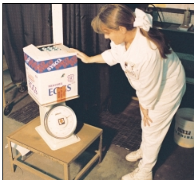
Figure 30. Bulk packages of eggs are check weighed on platform scales to verify minimum net weight. Test weights are used to verify the accuracy of the scale. (00-CN-0603)
