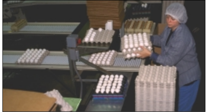
Figure 20. Packaged eggs leaving automatic packaging equipment are placed into shipped cases. (CD 8202 3241 1143-32)
