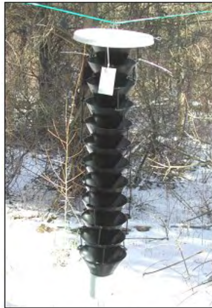
LINDGREN FUNNELTRAP FOR Sirex noctilio
