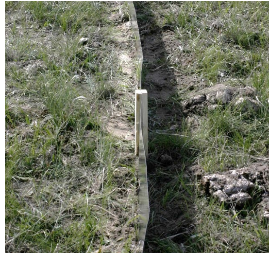
Figure 31. Drift fence made of aluminum flashing.
