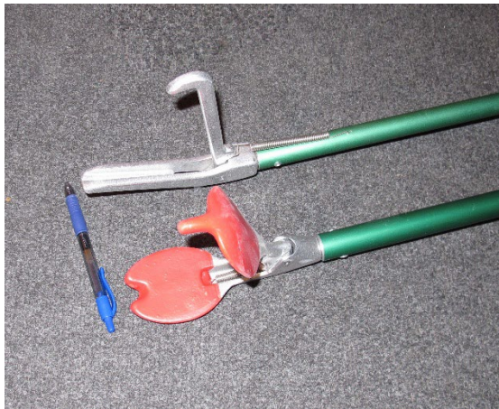
Figure 34. Narrow-mouthed tongs (top) and wide-mouthed tongs (bottom).
