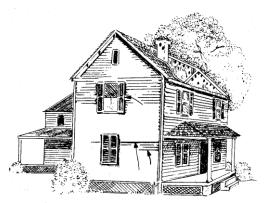
Figure 6. Potential bat roost sites in a structure.
