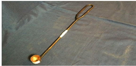
Figure 10. Bait dispensers can be made from copper pipe, split rivets, washers, and 1/4-inch rod. Match the capacity of the cut pipe with a baker's teaspoon. Label the dipper for pesticide use only.
