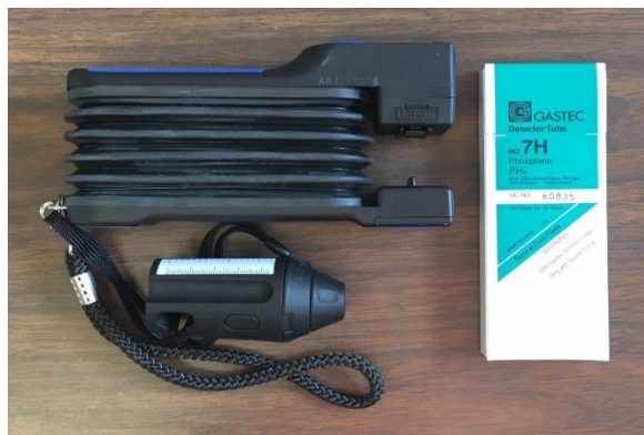
Figure 9. Hand-pump used to draw air into the glass testing tubes containing a chemical sensitive to the presence of phosphine gas.
