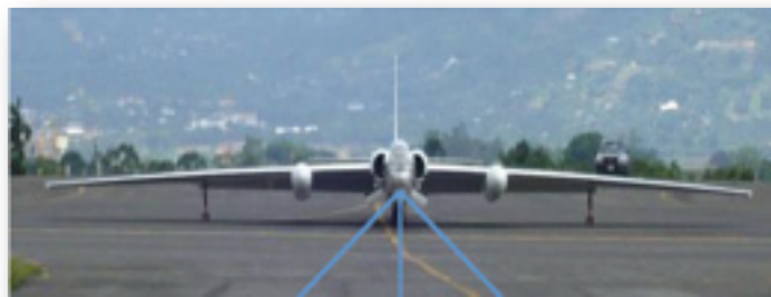
Fig. 35. ER-2 carrying MABEL in the nose, and indicating the instrument swath width.
