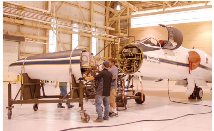
Fig. 34: The ER-2 crew rolls the aircraft's nose, containing MABEL, away from its body, so engineers can work on the instrument. (Credit: Kate Ramsayer, NASA)
