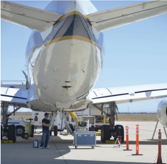
Fig. 33: Stewart Wu (GSFC) stands watch during ground-based laser testing outside hangar 703 of NASA Armstrong’s Science Aircraft and Integration Facility in Palmdale, CA. The laser beam is emitted nadir from the DC-8 aircraft and is redirected by the circular mirror atop the blue box. These tests ensure alignment of the transmit beam and receiver optics before the rigors of flight.
