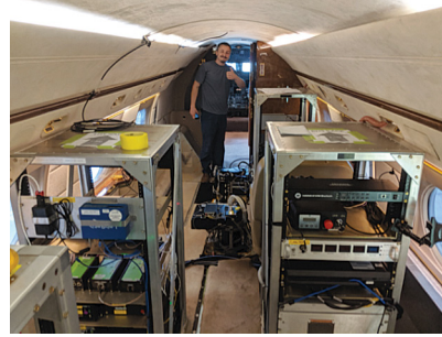
Image Right: LVIS lidars installed over the nadir optical ports along the centerline of the G-V, along with LVIS Engineer Shane Hendry. Photo credit: David Rabine
