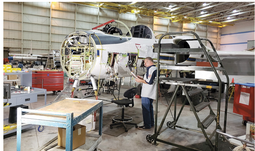
Bobby Henderson, Avionics Technician with Vertex, verifying wire installation with drawing for ER-2 809 CARE modification. Photo Credit: Brian Hobbs
