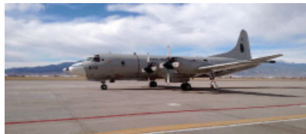
NRL P-3 (VXS-1 squadron, Pax River) deployed at Peterson AFB for SnowEx. Visible are NASA P-3's nose housing CAR and the tail & nadir housings for the SnowSAR.
