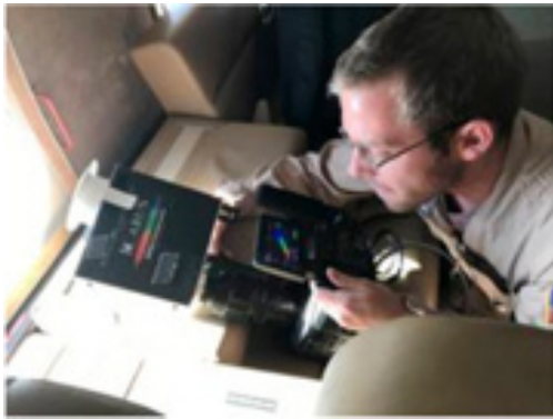
Armstrong videographer Mike Agnew tests spectrograph analyzing the sun's wavelengths for use on flight during the total eclipse. Credits: NASA Photo / Kevin Rohrer
