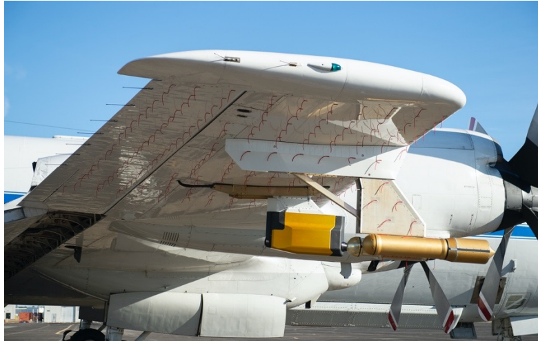
Tufts are attached on the wing and pylon for aerodynamic observation during test flights
