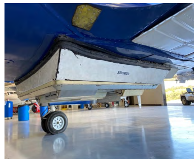
The AirSWOT instrument was flown onboard a Dynamic Aviation King Air aircraft. Photo credit: Roger Chao
