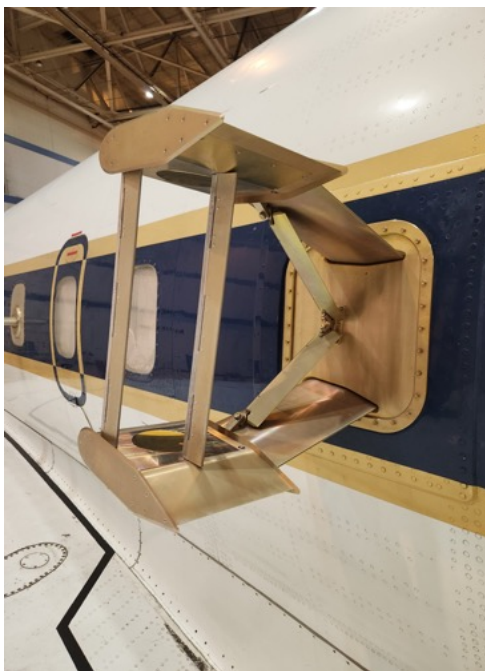
The OPALS instrument seen from the exterior of the DC-8. Note the metering rods and spherical mirrors seen in the image. Photo credit: Adam Webster
