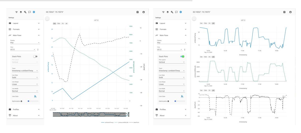
MTS Users can directly monitor real time aircraft housekeeping status and instrument status packets graphically with a variety of plot options.
