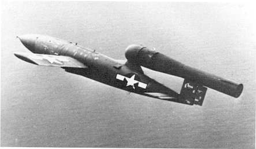
Test flight of the JB-2, an American copy of the German V-1.
