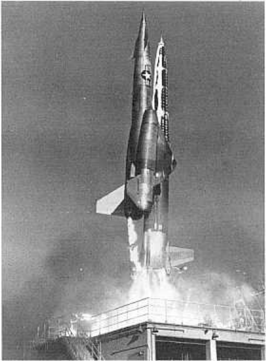
A Navaho cruise missile test-launched. The piggyback arrangement would be used years later by the space shuttle.
