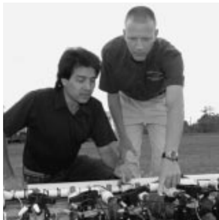
Cardenas-Lailhacar and Dukes check flowmeters used to monitor irrigation volume applied to turf grass research plots.
