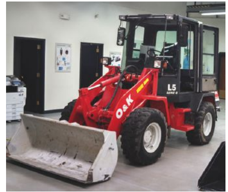
Prototype test vehicle with DC steer-by-wire system.
