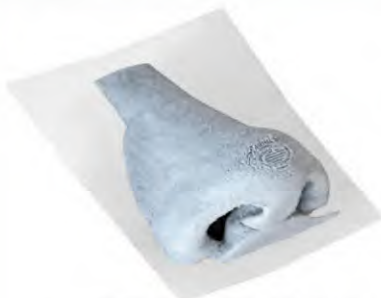
Silicone model printed on the 3D-Bioplotter from scan of a patient's nose.
