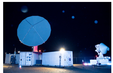
The NASA S-band NPOL (left) and Ka/Ku band D3R (right) dual-polarization Doppler radars installed on Quinault Nation land near Taholah, WA, in OLYMPEX.
