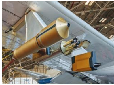
Three of the microphysics probes mounted on the wing of the NASA P-3. Photo courtesy of Victoria McDonald
