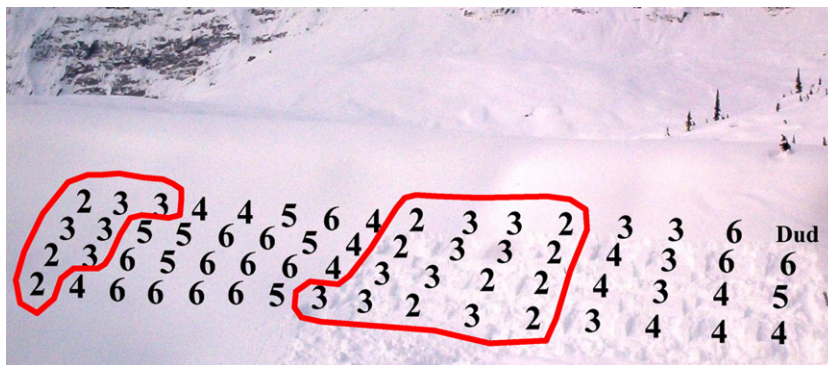
Fig. 2. Spatial array of point stability measurements on a small slope (Mt. Abbott, Columbia Mountains, western Canada) using the rutschblock test ( N=63 , spacing about 2.5 m, extent about 40 m). The slope median stability test score was 4 with a quartile coefficient of variation (QCV) of 50%. The slope shows distinct patterns of higher and lower stability. A similar pattern, though with some more variations, was found at this same site the following winter. The topography of the bare slope is characterized by cross-slope undulations. Campbell (2004) suggested that the observed stability was probably due to destruction of the surface hoar on higher ground by wind when the surface hoar was on the surface and subsequent preservation of the surface hoar in the more sheltered depressions (from Campbell, 2004, p. 89).
