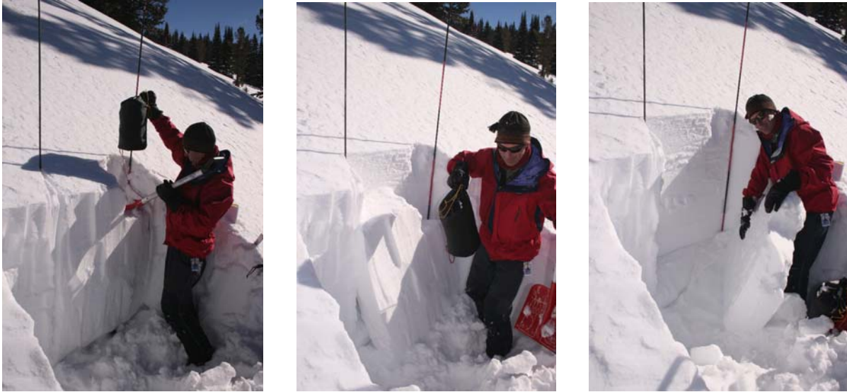
Figure 1: Though the ECT is typically loaded with the compression test loading steps, it can also be loaded using the stuffblock steps, as shown above. From left to right: loading the extended column, column fractures (ECTP), examining the fractured slab and weak layer. Photos by Jordy Hendrixx.
