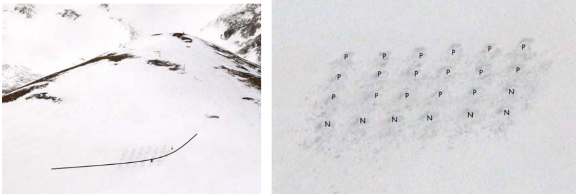
Figure 2: An overview of a grid of 24 pits on Tucker Mountain in Colorado. The black line in the photo at left marks the lower boundary of the hard slab involved in avalanches on similar slopes two days before our sampling. At right, a close-up of the grid showing the locations with ECTP results (shown as "P") and locations where the result was ECTN (shown as "N"). An active slab existed only at the upper left part of the grid, which is clearly reflected in the ECT results.
