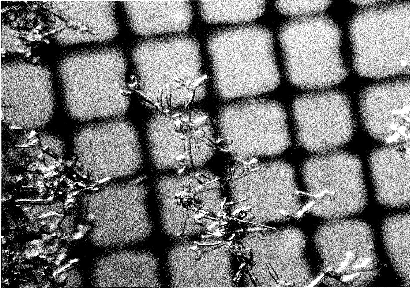
Figure 4.5: A 2 mm broken precipitation particle harvested from the surface of the south-facing study site on 10 January 2004. This crystal is classified by Colbeck et al. (1990) as type 2a/b.
