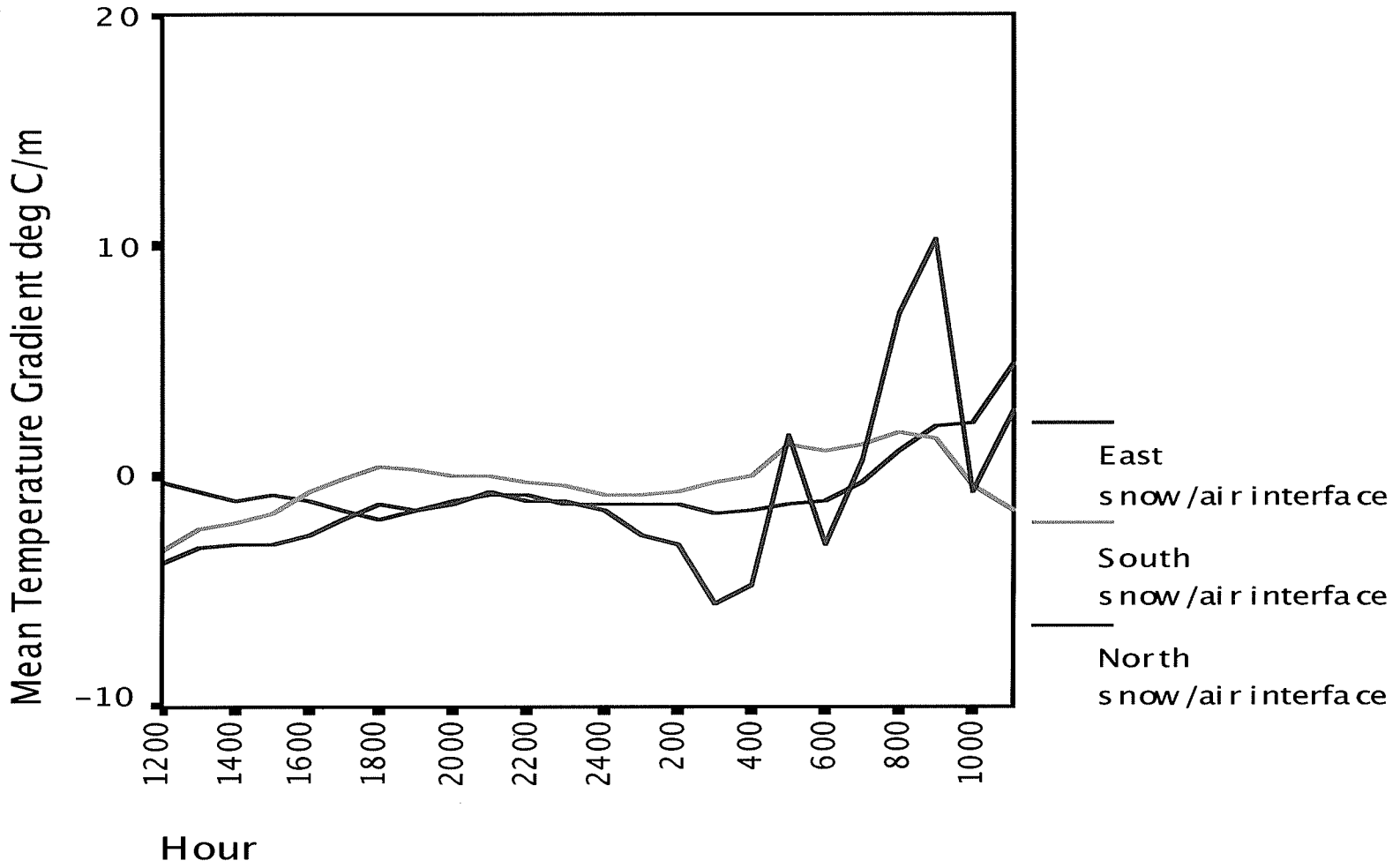
Figure 4.23: The mean temperature gradient by hour from 1200 hours on 23 January 2004 to 1100 hours on 24 January 2004 on the east facing, south facing, and north facing aspects at the snow/air interface.
