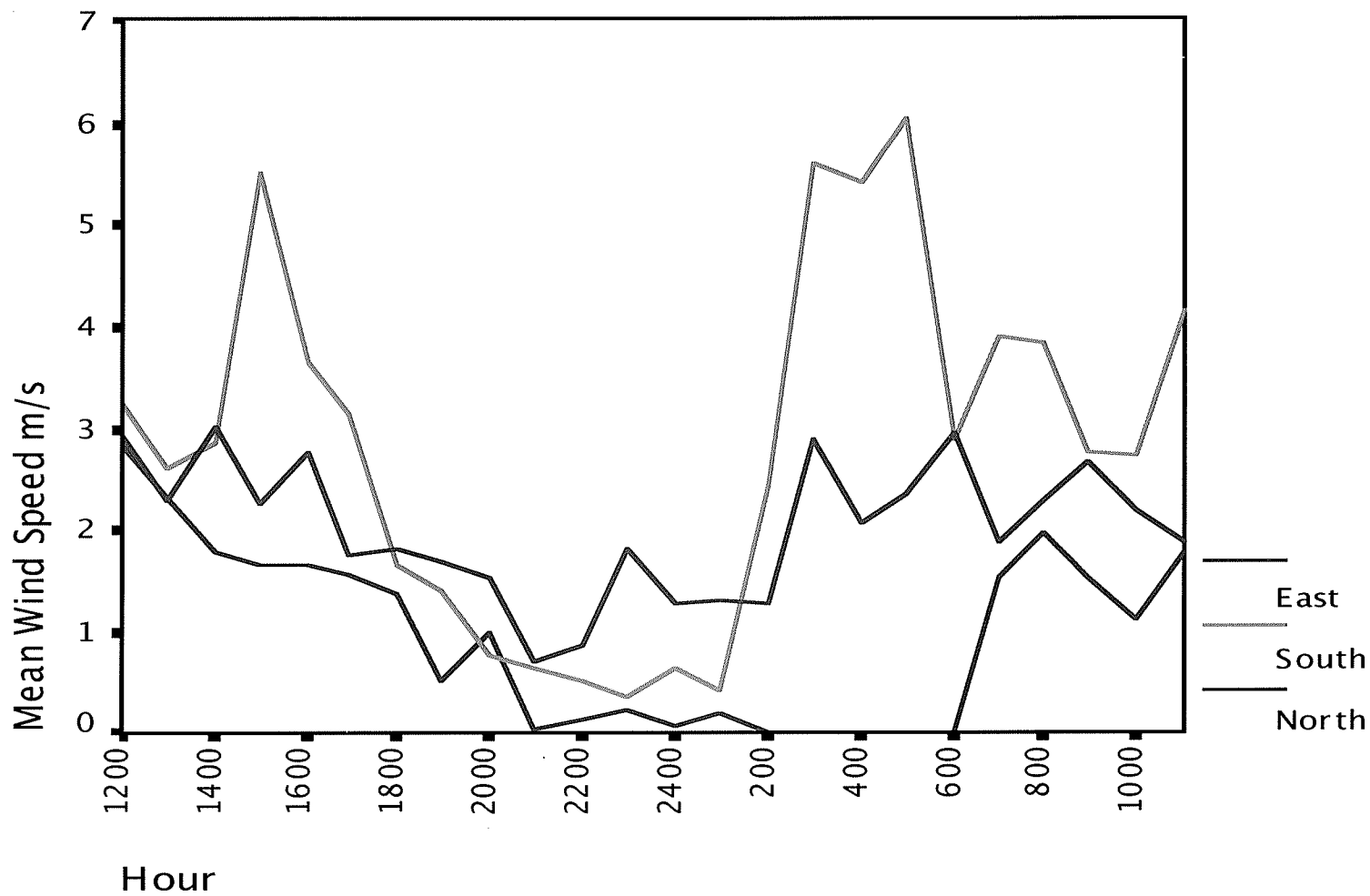
Figure 4.26: The mean wind speed ( \text{m s}^{-1} ) by hour from, 1200 hours on 23 January 2004 to 1100 hours on 24 January 2004 on north-facing, south-facing, and east-facing aspects.
