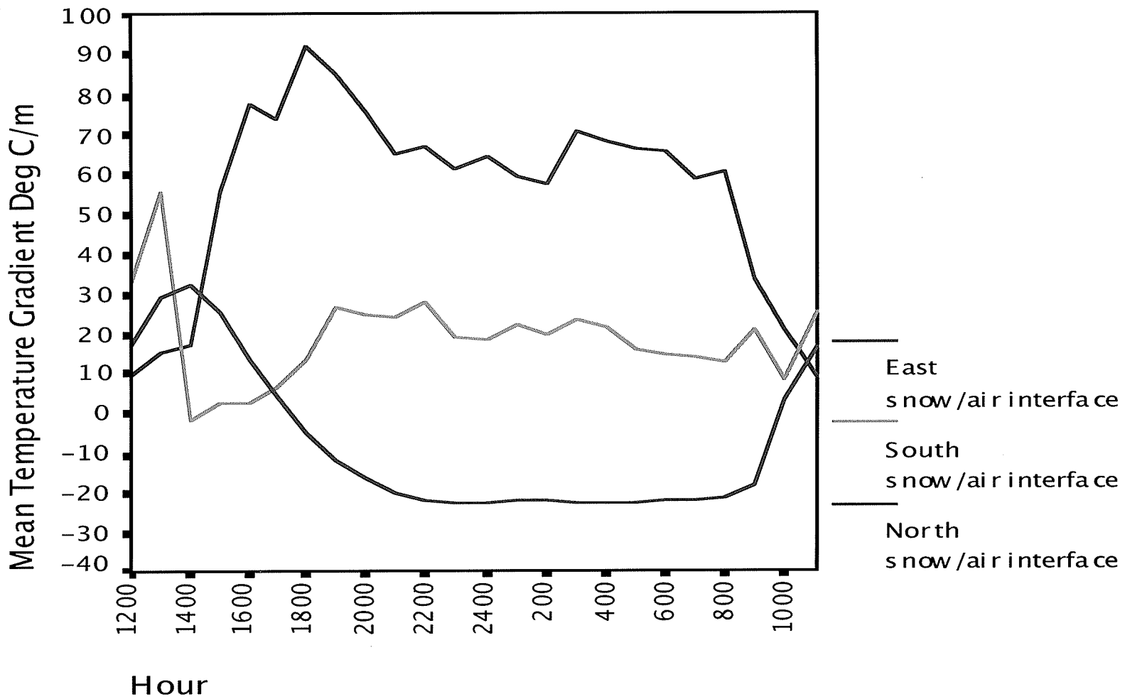
Figure 4.6: The mean temperature gradient by hour from 1200 hours on 9 January 2004 to 1100 hours on 10 January 2004 on the north-facing, south-facing, and east-facing aspects at the snow/air interface.
