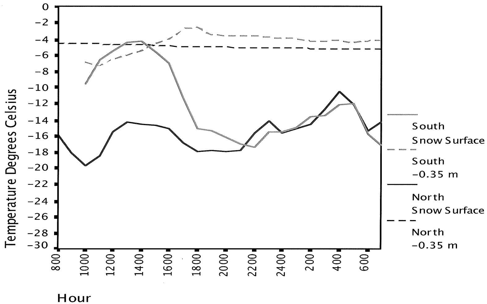
Figure 4.41: The snow surface temperature and the temperature at -0.35 m ( ^{\circ} C) by hour from, 0800 hours on 21 January 2004 to 0700 hours on 22 January 2004 on north-facing and south-facing aspect.
