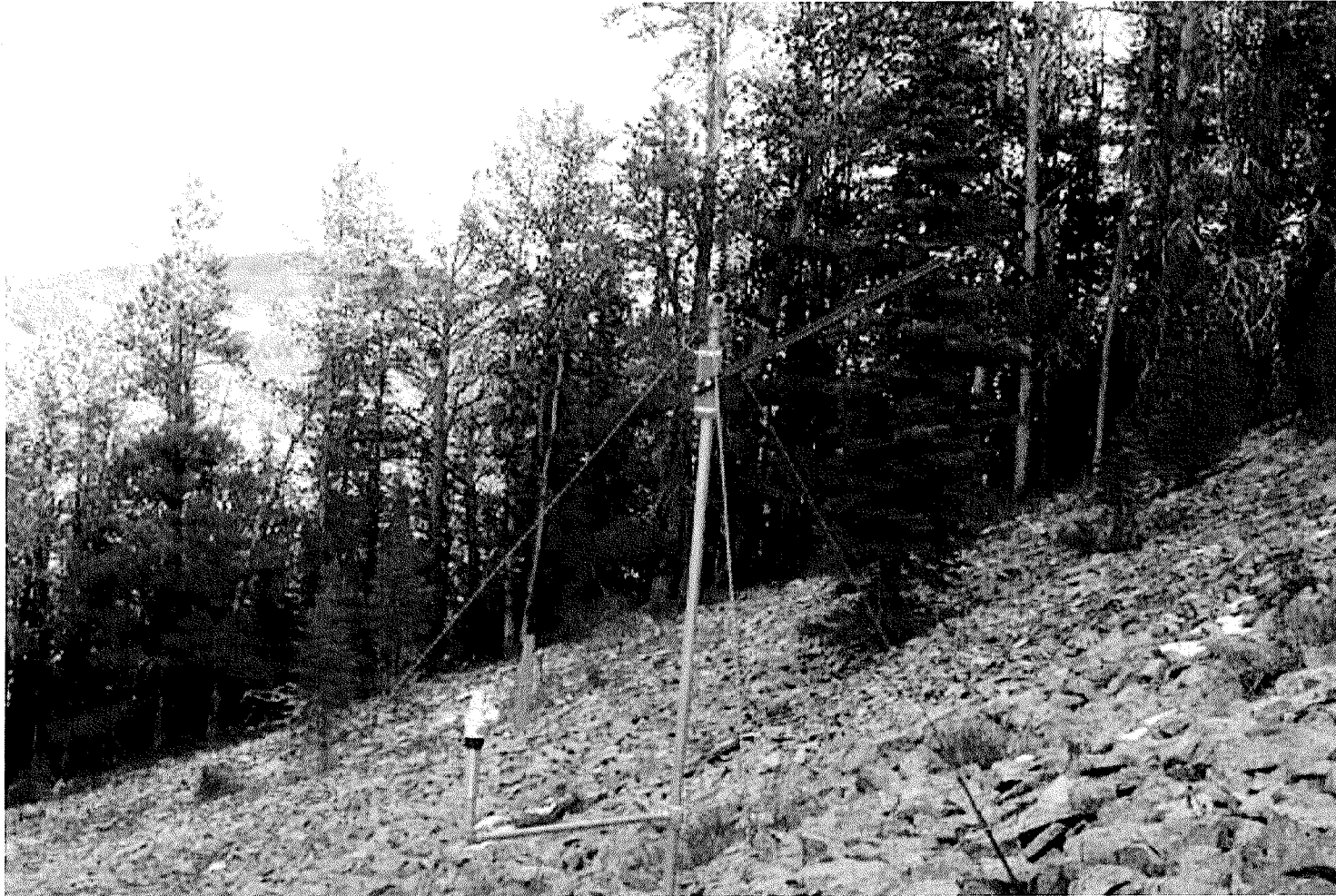
Figure 3.4: The north study site in the summer time. It clearly shows the scree slope, the movable anemometer, and the pyranometers mounted on the arm at the top of the photograph.
