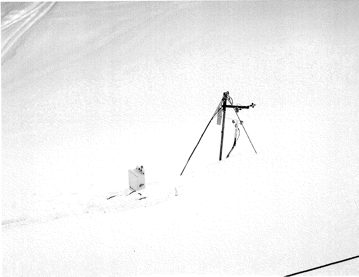
Figure 3.5: The north study site in the winter, showing the anemometer with its movable arm and the pyranometers. Also in view are the datalogger and the thermocouple array (center of photograph).
