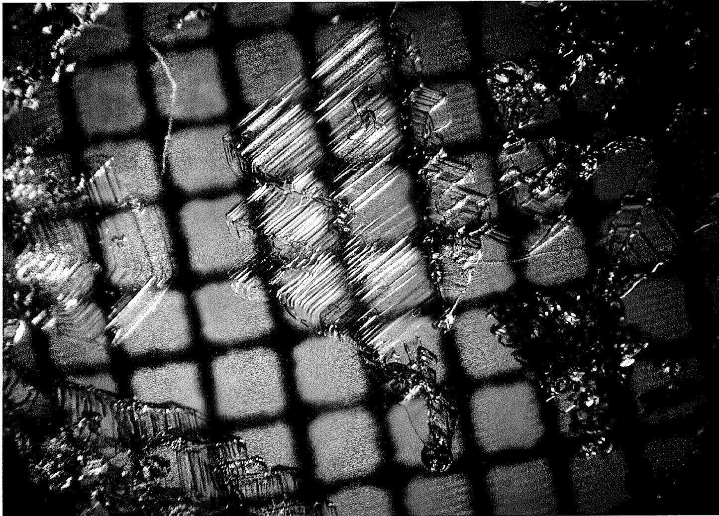
Figure 4.1: A 6mm surface hoar crystal harvested from the north-facing site on 10 January 2004. This crystal is classified by Colbeck et al. (1990) as type 7a.
