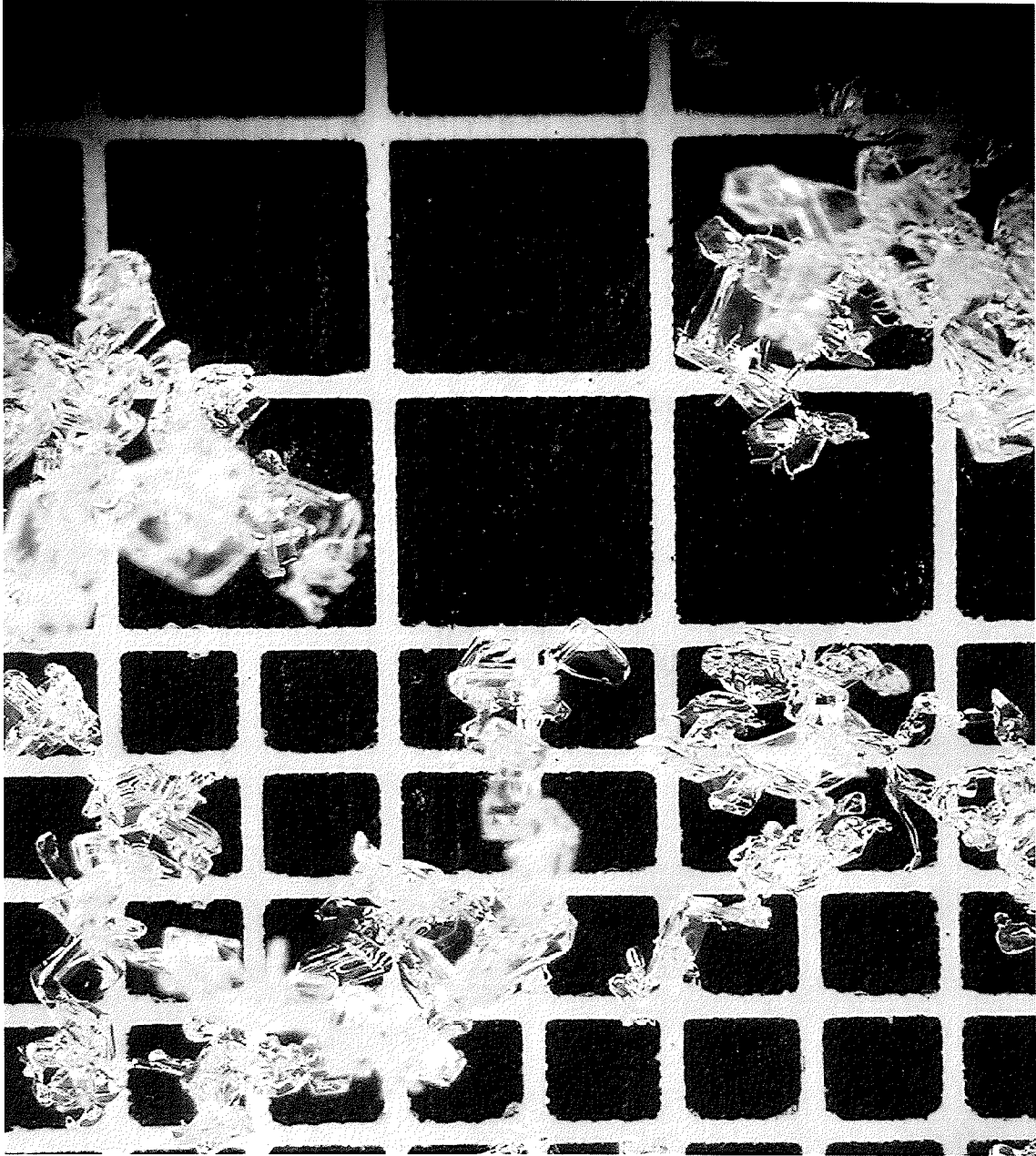
Figure 4.37: A few 1 mm near-surface faceted crystal harvested from the east-facing study site on January 22, 2004. These crystals are classified by Colbeck et al. (1990) as type 4a, solid faceted particles.
