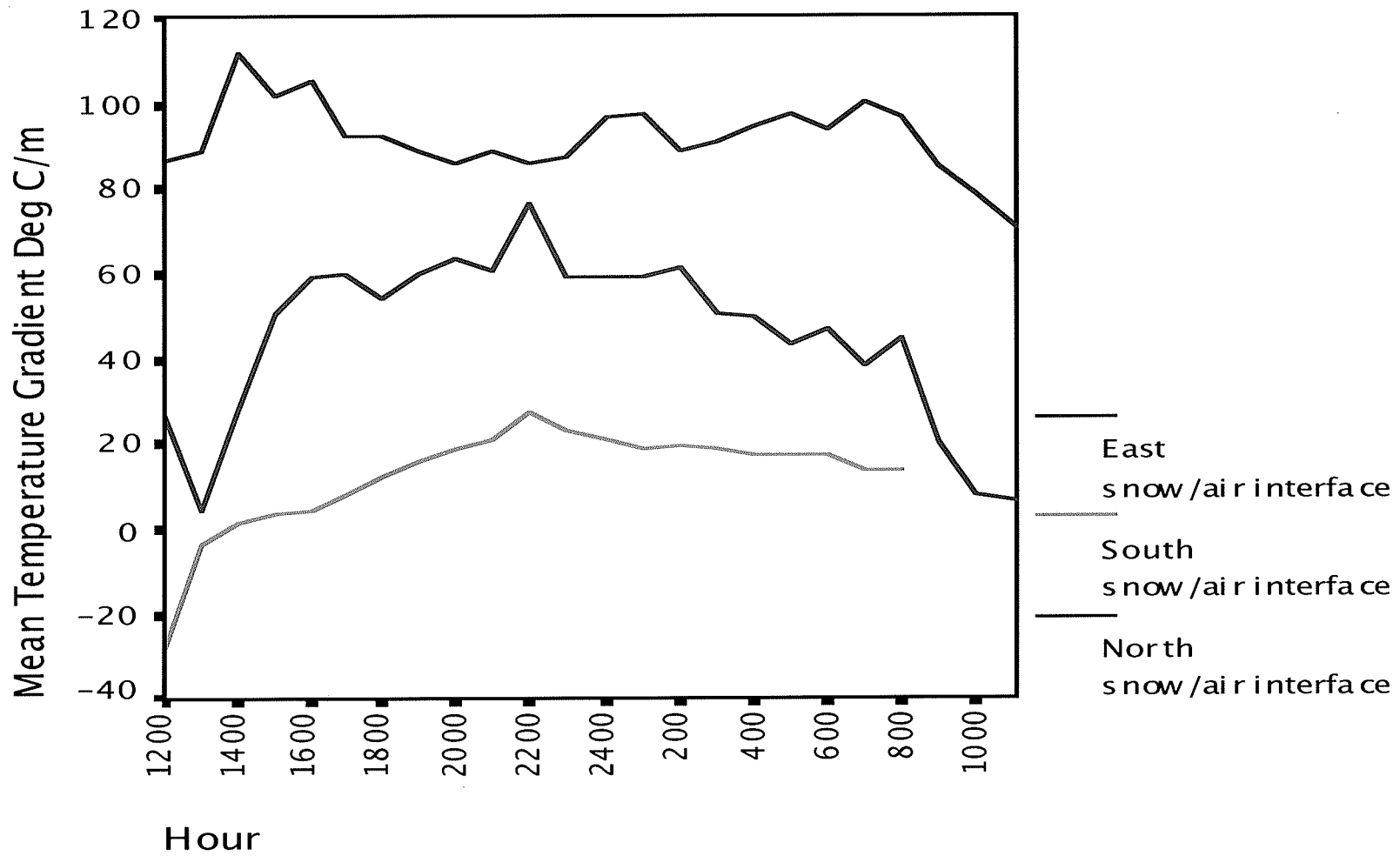
Figure 4.17: The mean temperature gradient by hour from 1200 hours on 12 January 2004 to 1100 hours on 13 January 2004 on the north-facing, south-facing, and east-facing aspects at the snow/air interface.
