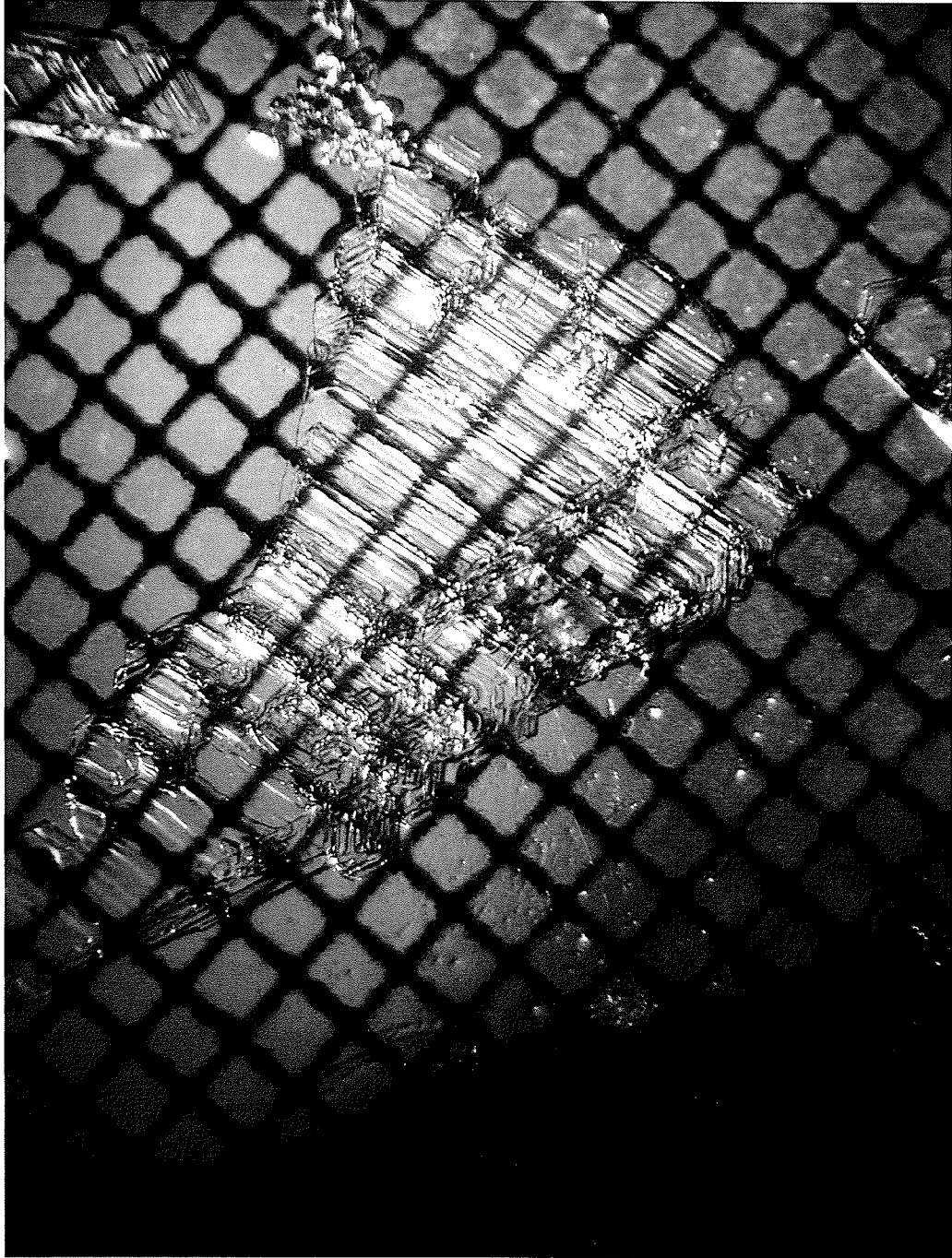
Figure 4.13: A 11mm surface hoar crystal harvested from the north-facing study site on 13 January 2004. This crystal is classified by Colbeck et al. (1990) as type 7a.
