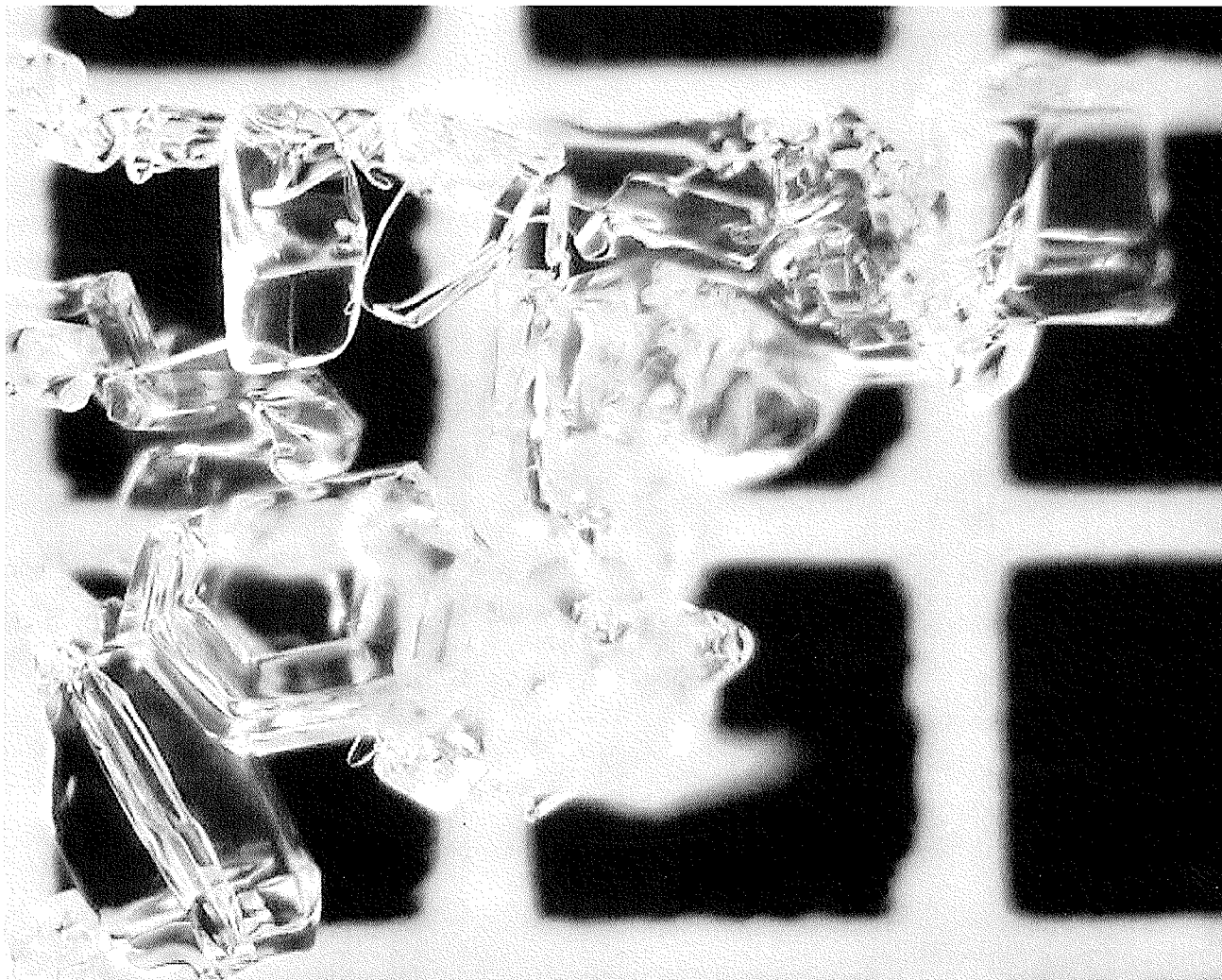
Figure 4.42: One mm faceted crystals harvested from the north-facing study site on 13 March 2004. These crystal would be classified by Colbeck et al. (1990) as type 4a, solid faceted particles.
