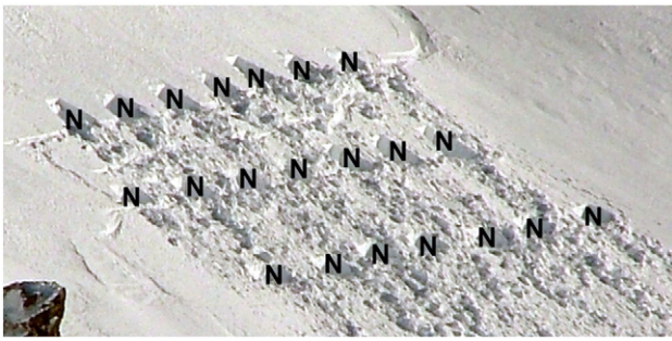
Fig. 3. ECT results from 21 pits on a stable 32° slope at Mount Hutt range in New Zealand. None of the tests propagated across the entire column (ECTN).
