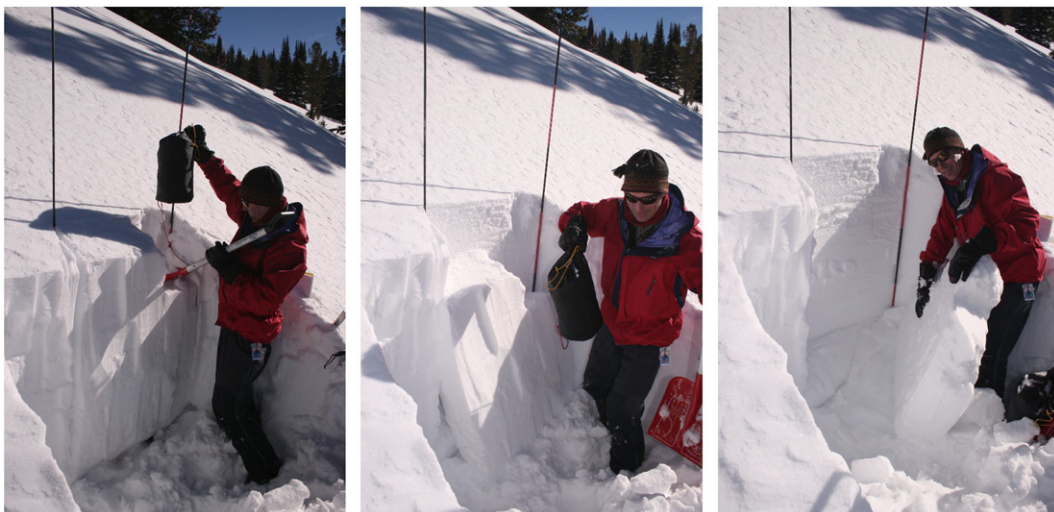
Fig. 2. Though the ECT is typically loaded with the compression test loading steps (Greene et al., 2004), it can also be loaded using the stuffblock steps (Birkeland and Johnson, 1999), as shown above. From left to right: loading the extended column, column fractures ( ECTP ), examining the fractured slab and weak layer. Photos by Jordy Hendrikx.
