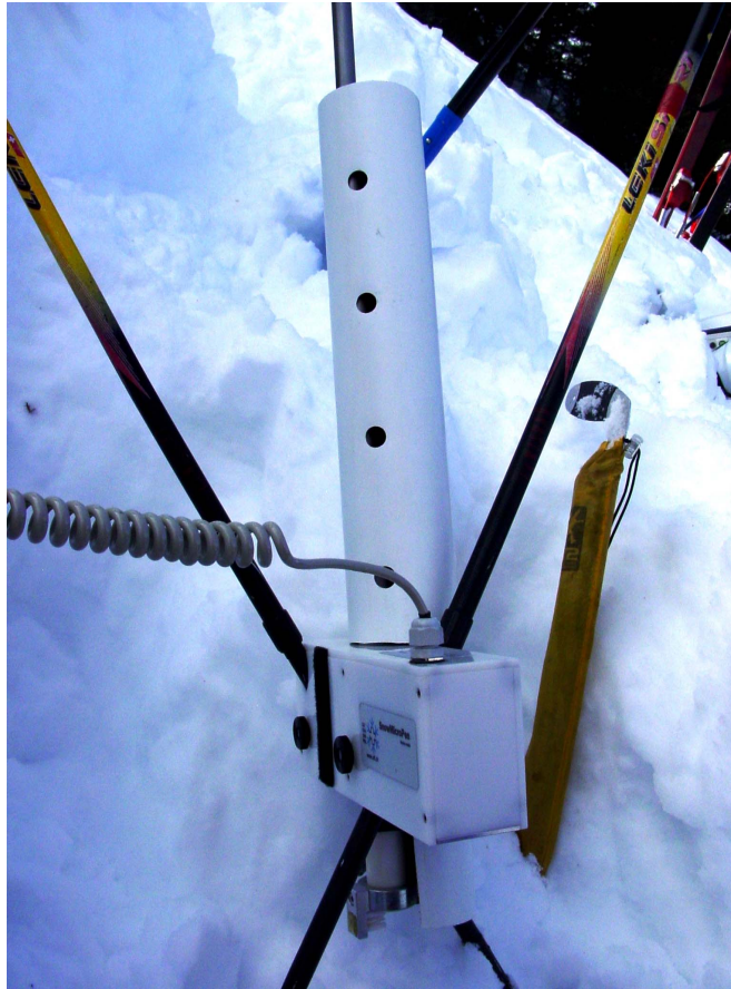
Figure 18. SMP retro-fitted with PVC packing container, which doubled as a shading device, as well as adjustable ski poles which aided in long reaches.
