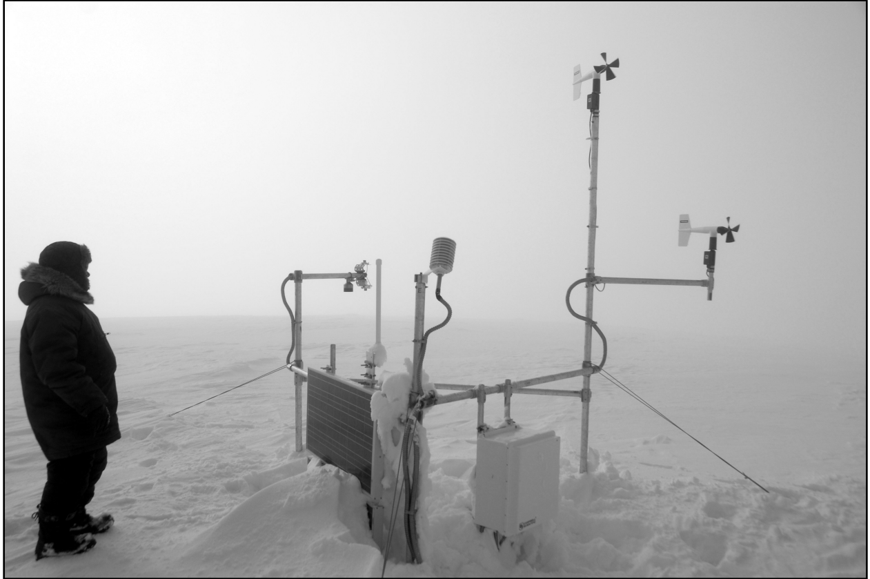
Figure 12. Ilkoo Angutikjuak examines the Akuliaqattak Station ( 70^{\circ}18'50''\text{N} , 68^{\circ}9'24''\text{W} ) in near whiteout conditions. Note temperature/relative humidity sensor on center leg, which has been bent by a visiting polar bear. Two such bear incidents have fortunately not compromised measurements.
