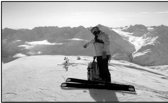
Figure 16. Nick Houfek points to the anemometer after a heavy snowfall season in the Chugach. The leg will be extended vertically to accommodate extreme snow depths.
