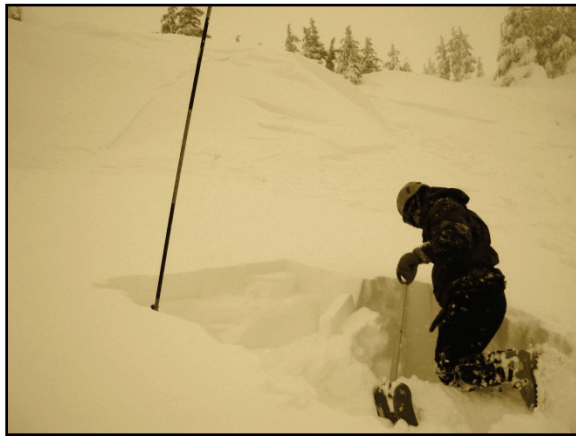
Figure 2: Dataset 1 test area. Obvious signs of instability are visible in the background. When we tried to sample a day later, weak snowpack layer fractures arrested before crossing our ECT columns (ECTN).
