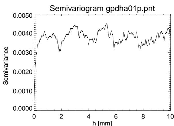
Fig. 7: Semivariogram with unfiltered force signal of faceted, temperature gradient metamorphosed snow.
