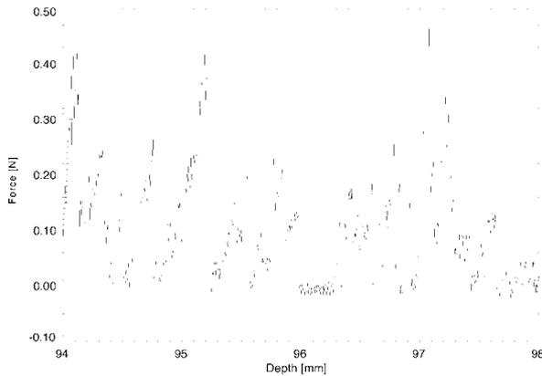
Fig. 3: Force signal measured in faceted temperature gradient metamorphosed snow.
