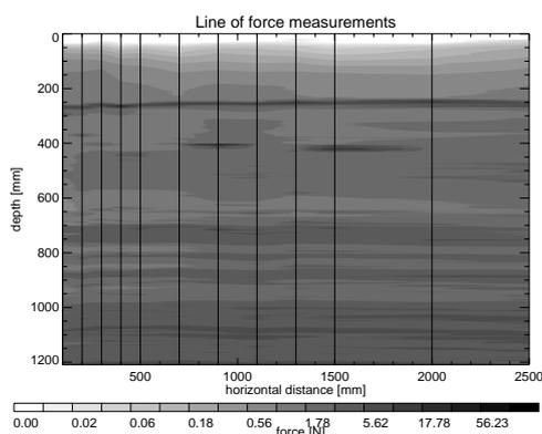
Fig. 13: Visualisation of two-dimensional spatial variability of a line of penetrometer snow profiles.
