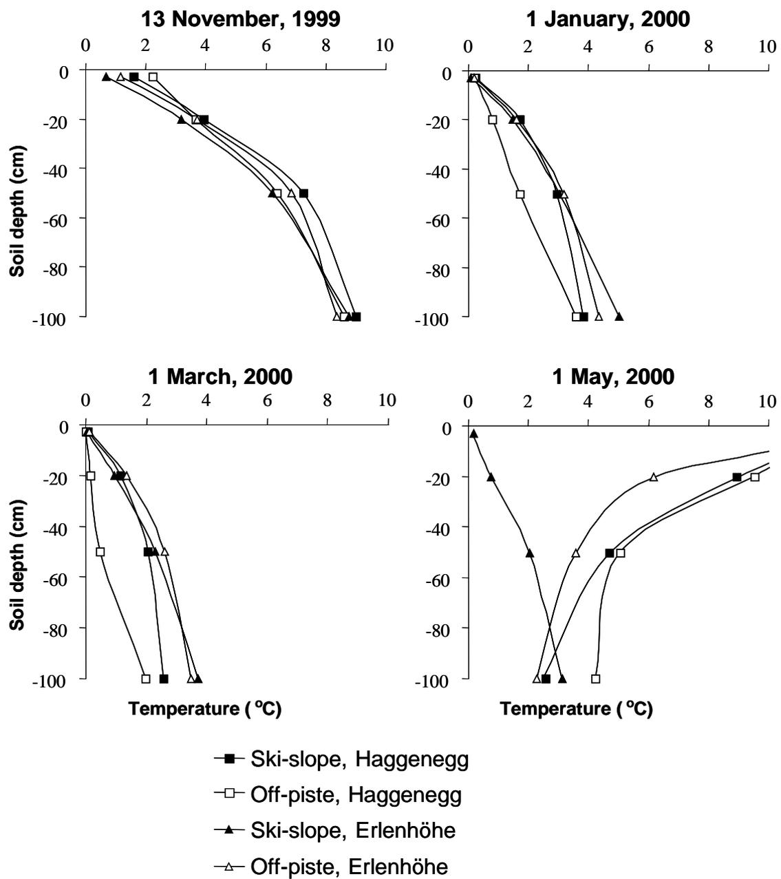
Fig. 4: Measured soil temperature profiles (°C) at four representative dates during the winter 1999/2000.
