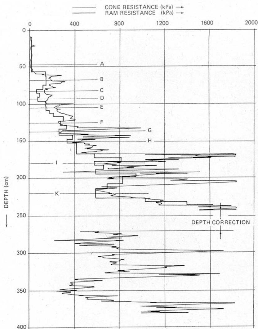
Fig. 18: Cone penetrometer hardness profile compared to ram hardness (Schaap und Föhn, 1987). The cone penetrometer resolves more layers and greater hardness variation in the snow profile than the ram test.
