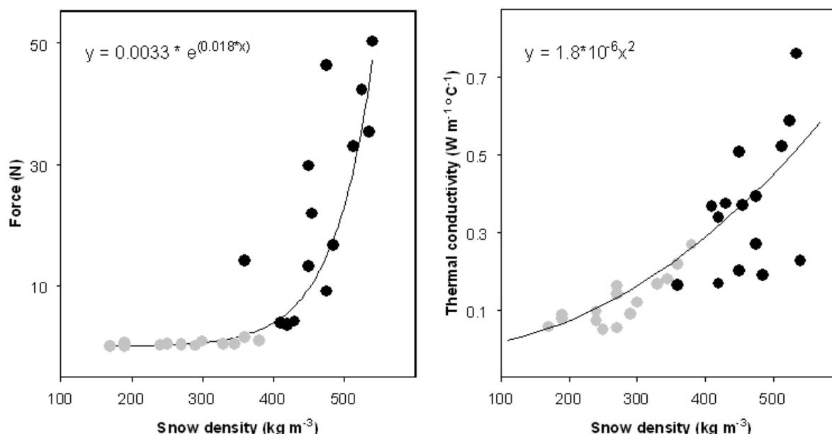
Fig. 3: Relationship between snow density ( $\text{kg m}^{-3}$ ) and snow hardness (N, left), as well as thermal conductivity ( $\text{W m}^{-1} \text{ }^\circ\text{C}^{-1}$ , right) measured on 12 January on the ski-slope (dark dots) and in the natural snowpack (light dots).
