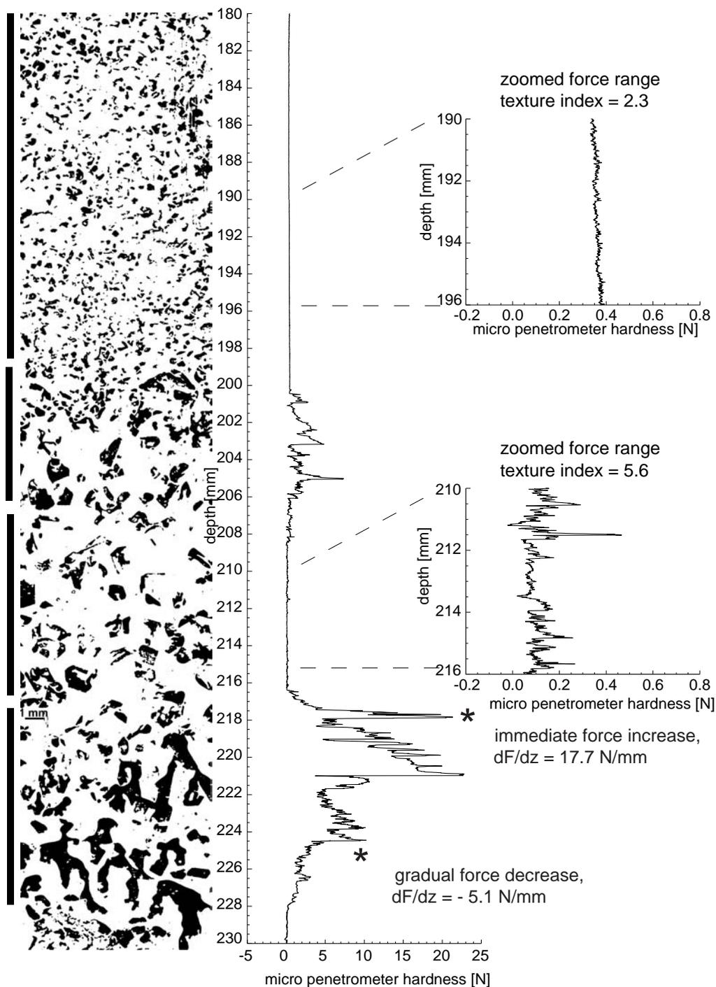
Fig. 2: Snow profile from 9 Jan. 2002: serial sample containing two crusts (black is ice). The black vertical bars on the left mark the layers as they are depicted from the surface image. Their interruptions mark the layer boundaries. This is an example where the stratigraphy established by hand hardness agrees with the surface image. Snow texture and hardness gradients at layer boundaries are calculated from the micro penetrometer hardness signal.
