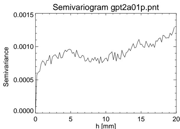
Fig. 6: Semivariogram with filtered force signal and reduced variance (for round-grained, equi-temperature metamorphosed snow).
