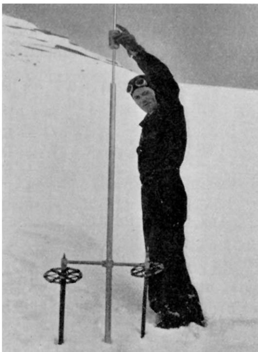
Fig. 8: Swiss Ramsonde was developed by Haefeli (Bader, Haefeli et al., 1939) to obtain an objective mechanical hardness profile of the snowpack.
