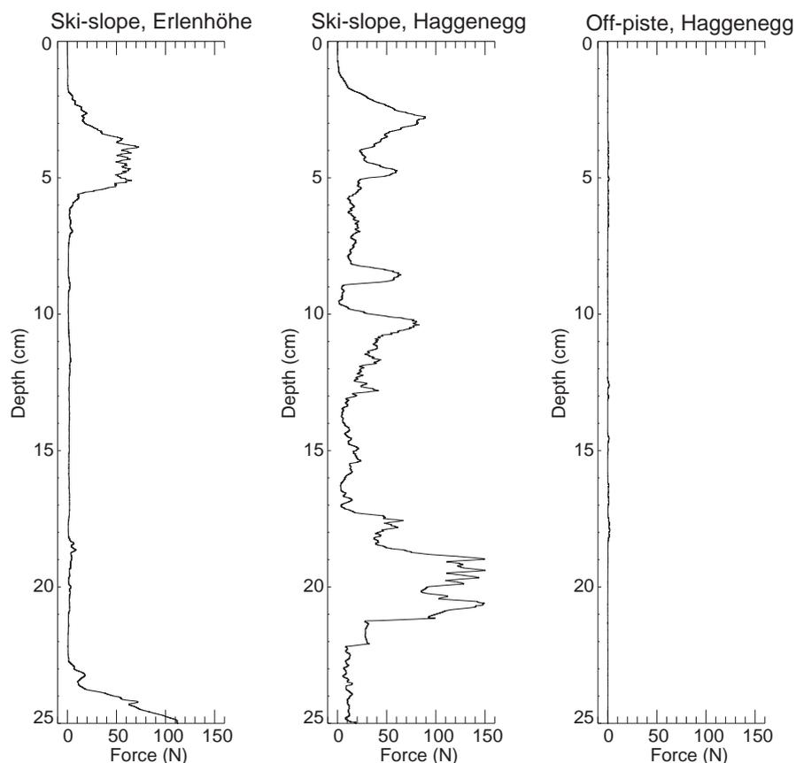
Fig. 2: Examples of penetration force signals measured with the Snow Micro Pen on 12 January, 2000 at three locations of the ski resort Brunni-Haggenegg: (left) ski-slope Erlenhöhe, (centre) ski-slope Haggenegg, and (right) off-piste Haggenegg.
