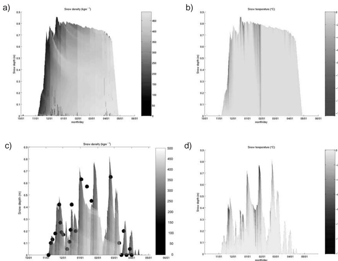
Fig. 5: Simulated snow density profile (left) and snow temperature profile (right) for the ski-slope (top) and the off-piste (bottom) site Haggenegg. For the off-piste site, measured snow depth is indicated with black dots.
