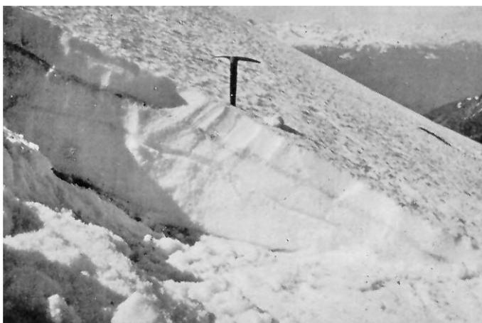
Fig. 5: “A snow section where two crust layers between the three snow strata are clearly seen (see Fig. 6, A). If the ice layers are frozen to the snow strata, there is no danger of the snow sliding off by strata.”: (Seligman, 1936, p. 310)
