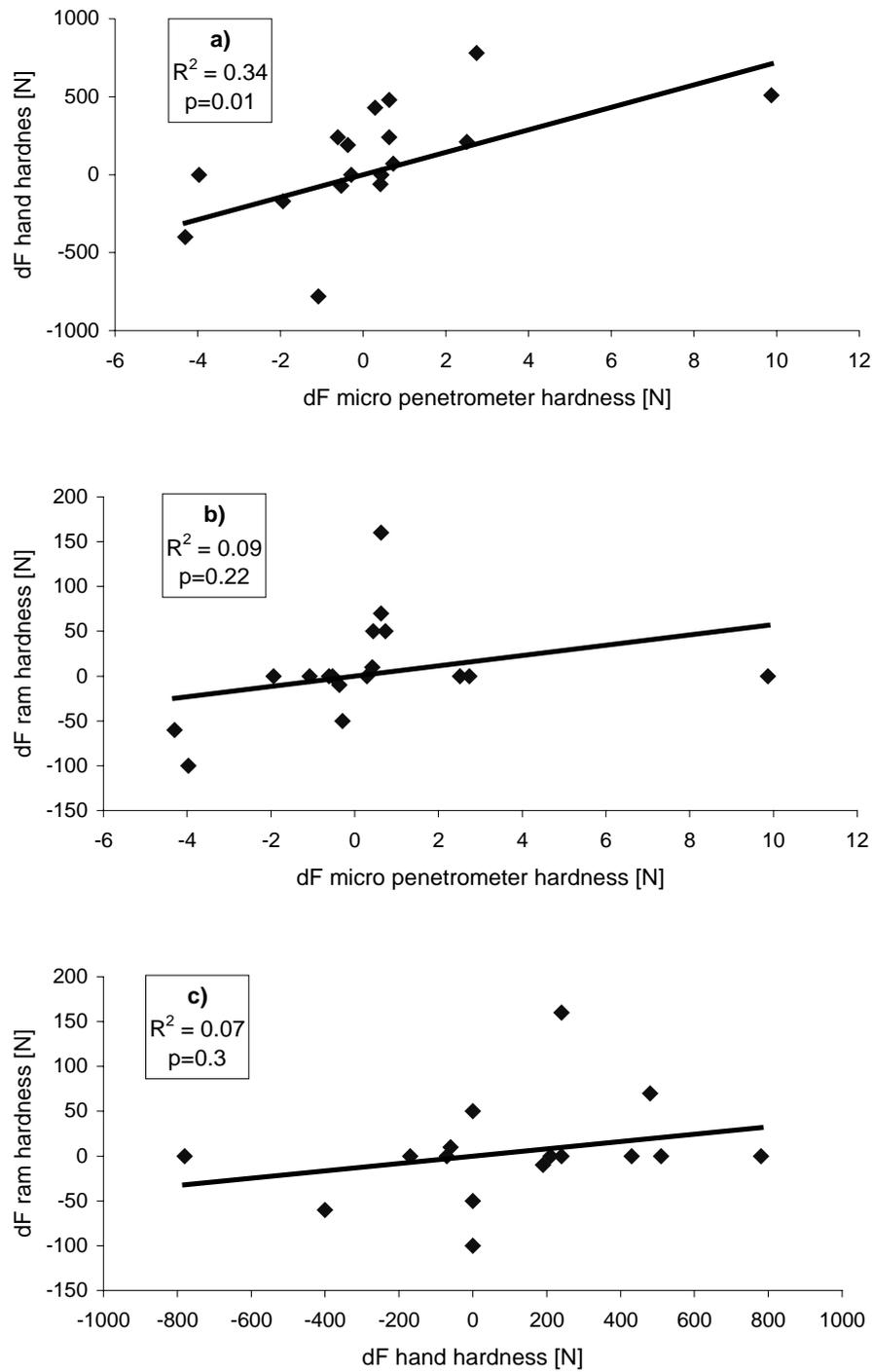
Fig. 5: The hardness differences (dF) at layer boundaries between: a) hand and micro penetrometer hardness are correlated ( $p=0.01$ ), b) ram and micro penetrometer hardness and c) ram and hand hardness are uncorrelated ( $p$ -values at 95 % confidence level).
