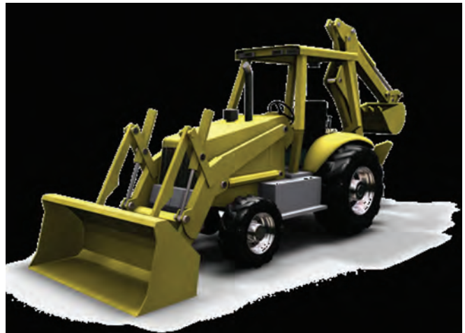
Figure 3. Backhoe facet model used in Xpatch scattering predictions
