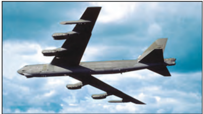
Figure 2. B-52H with concept wingtip jamming pods (image by Guy Aceto)
