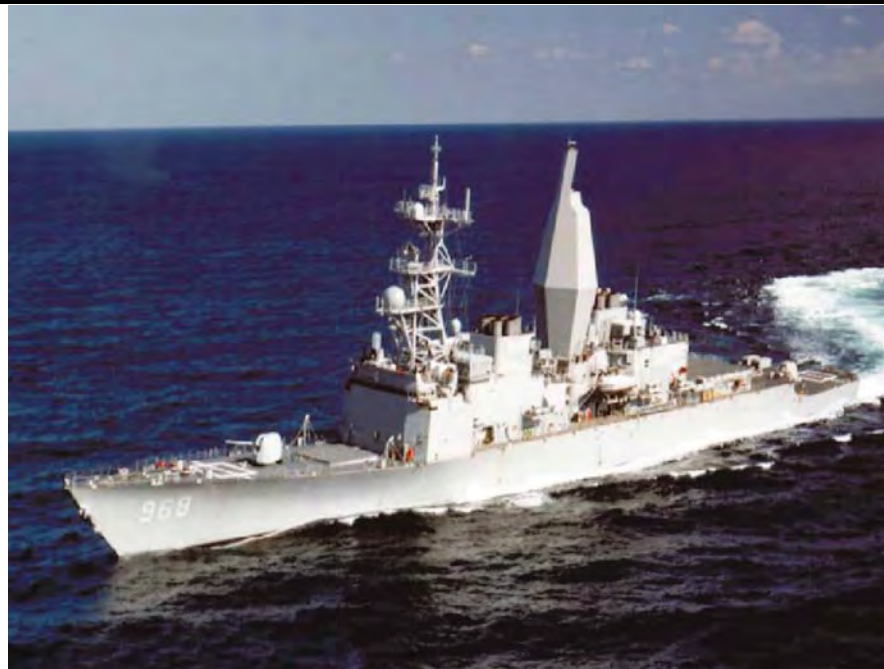
Figure 1. USS Radford with Advanced Enclosed Mast/Sensor (AEM/S) mast. (Courtesy U.S. Navy and Space and Naval Warfare Systems Center, San Diego)
