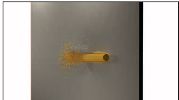
Impact of a uranium alloy rod on an aluminum plate
