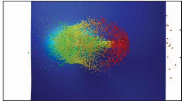
Impact of a uranium alloy rod on an aluminum plate, colored by pressure
