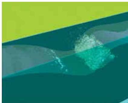
Figure 3. Overview of the plunging wave breaking over a submerged bump
