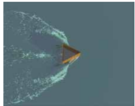
Figure 1. Wave breaking around a wedge-shaped bow
