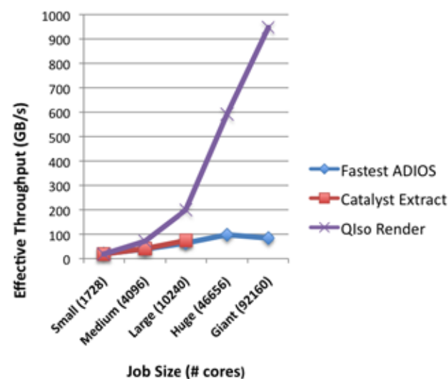
Figure 2. Effective throughput for the two coprocessing methods as compared to fastest I/O methods.
