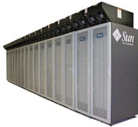
Midnight is ARSC's 2312-processor Sun Opteron cluster with a 68-TB Lustre file system
