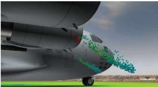
The pulse jets device uses high-pressure air to alternatively eject fluid from two nozzles mounted underneath the engine nacelle close to the nacelle lips. The intermittent high-frequency ejection provides turbulent mixing to prevent the formation of a coherent vortex. The particles are colored from 0.5 Mach (red) to 0.0 Mach (blue)
