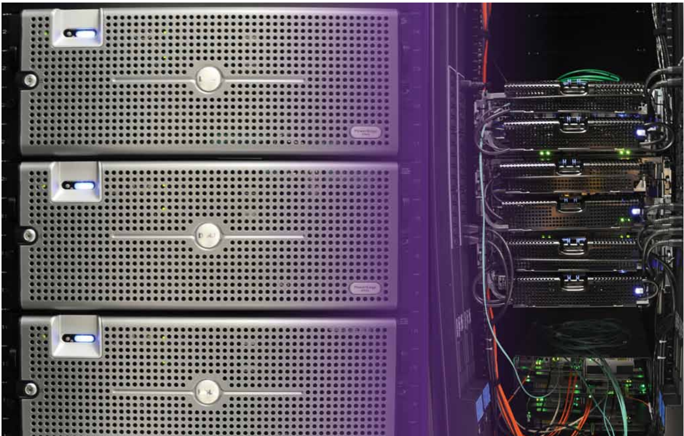
Front and back image of the three esLogin nodes installed on Pingo , a Cray XT5 at ARSC DSRC
