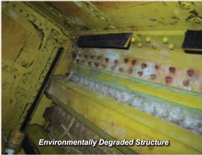
Figure 1. C-130 center wing box with service-induced damage
