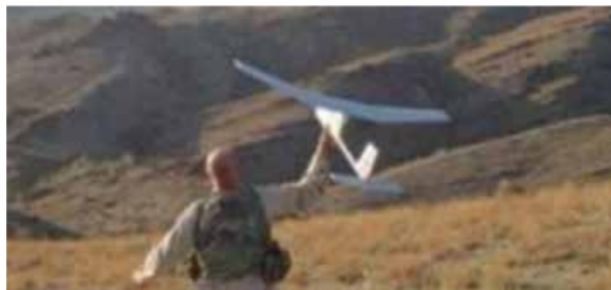
AeroVironment RQ-11 Raven is a small hand-launched remote-controlled unmanned aerial vehicle (or SUAV).
