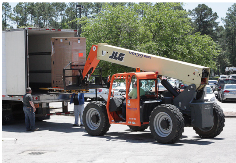
A telehandler forklift unloading a carefully packaged cabinet for the Navy DSRC Cray XC30 system Armstrong.
