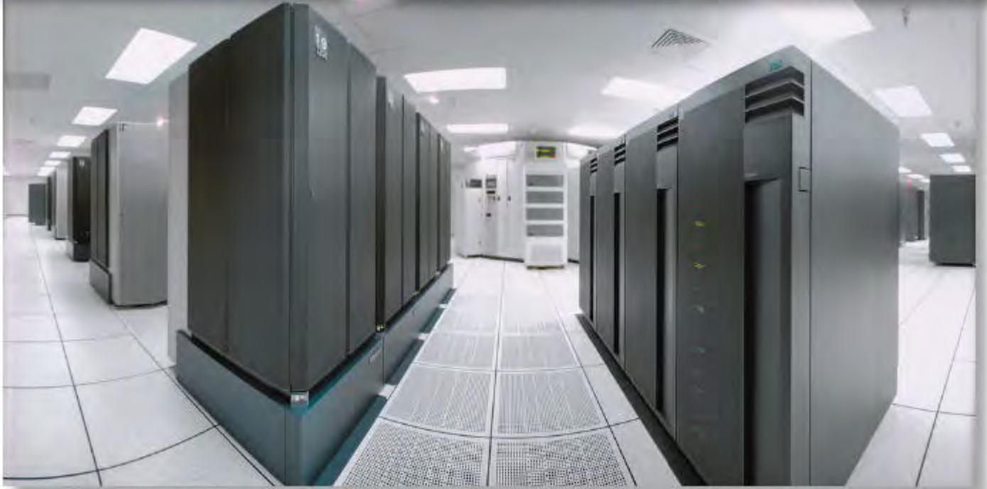
NAVO MSRC recently completed installation of an IBM RS/6000 SP supercomputer, code named "Habu." One of the largest systems ever built by IBM, Habu cruises at over 2 trillion operations per second, making it one of the fastest and most capable HPC systems in the world today. TOP LEFT: Unloading one of the two moving vans needed to transport the components. TOP RIGHT: Technicians begin installing the 24 cabinets that house the computer. BOTTOM: A panoramic photo of the completed system.
