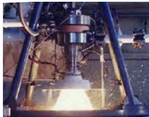
Figure 1. Systems representing external (X-15, above) and internal flows (Rocket nozzle, right) in thermal nonequilibrium (images taken from http://www.grc.nasa.gov/WWW/K-12/airplane/rocket.html ).
