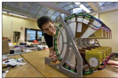
An arm of the T2 telescope, which uses gas electron-multiplier (GEM) chambers, under construction.
