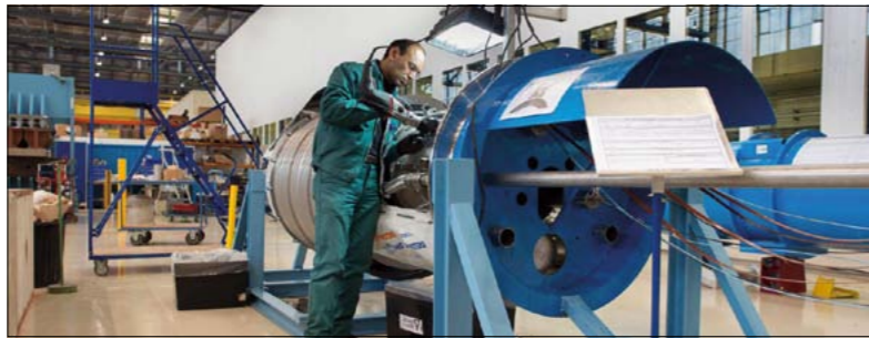
A technician practices opening a spare LHC magnet casing in CERN’s magnet-testing facility. During the long shutdown, 10,170 such casings will be opened to consolidate interconnections inside.
