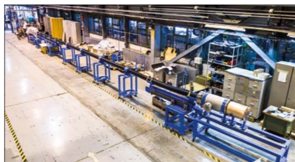
A semi-flexible cryostat (the black tube) for cooling MgB_2 cables undergoing testing in the new facility in SM18 at CERN. This tube is 20 m long and has a diameter of approximately 16 cm.
