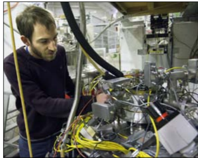
Stephan Ettenauer with the Penning trap apparatus that allows measurements of single antiprotons in the ATRAP experiment.
