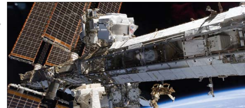
Perched on the International Space Station around 400 km above the Earth, the Alpha Magnetic Spectrometer (AMS) collects data from primary cosmic rays before they can interact with the atmosphere. (Image credit: NASA.)
