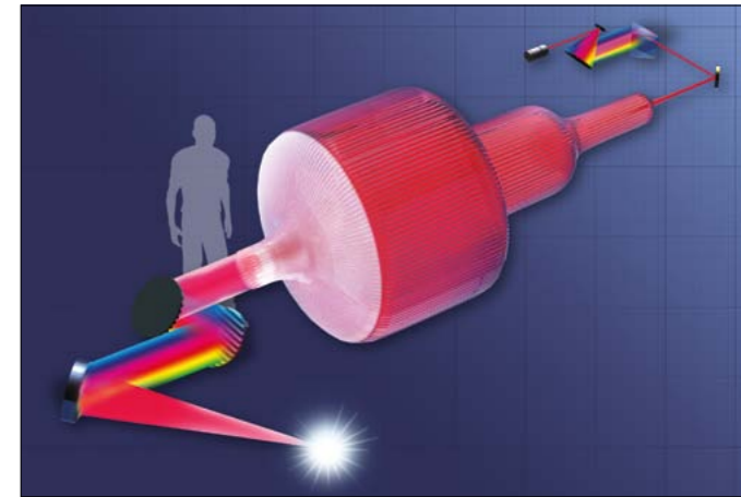
Fig. 1. The concept of the CAN fibre laser, in which an initial pulse from a seed laser is stretched and split into many fibre channels. Each channel is amplified in several stages and then combined coherently, compressed and focused to produce a pulse with >10J energy at a repetition rate of around 10kHz. (Image credit: Phil Saunders/spacechannel.org.)
