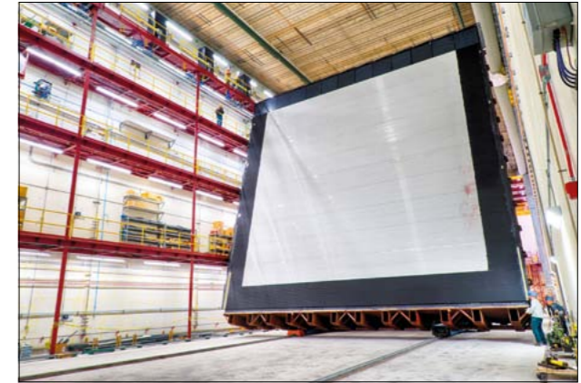
When completed, the NOvA far detector will comprise 28 detector blocks, each measuring about 15 m tall, 15 m wide and nearly 2 m deep. (Image credit: Fermilab.)
