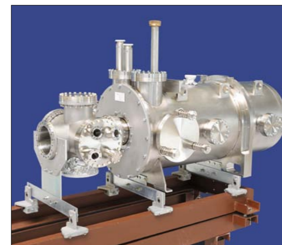
(Left) Fig. 3. A high-field 13 T magnet structure in Nb 3 Sn with dummy aluminium coil. (Image credit: J Muñoz Garcia and J-C Perez.) (Right) Fig. 4. A cryo-catcher prototype for the FAIR project. (Image credit: GSI.)
