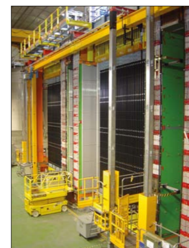
The OPERA detector, built from two identical super modules, each containing a target section and a large-aperture muon spectrometer. The target consists of alternate walls of lead/emulsion bricks – with 150,000 bricks in total – and modules of scintillator strips for the target tracker. (Image credit: OPERA.)
